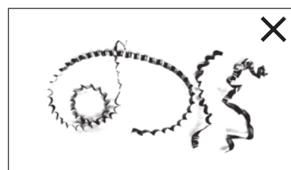
Continuously coiled long chips
