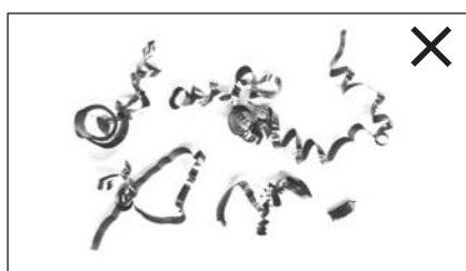
Apple-peel-like chips (Without curling)
