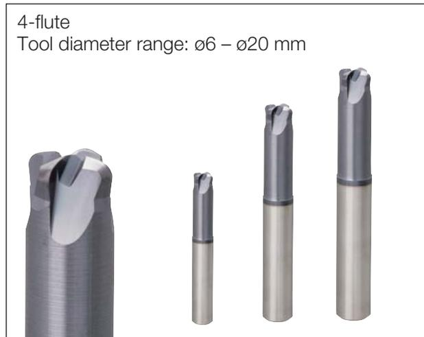
Due to this geometry, the solid **FeedMeister** can operate at feed per tooth ( $f_z$ ) rates up to 0.5 mm/z, at 0.3 to 0.7 mm depth of cut ( $a_p$ ), providing a significant reduction in cycle time, which thus increases productivity.
