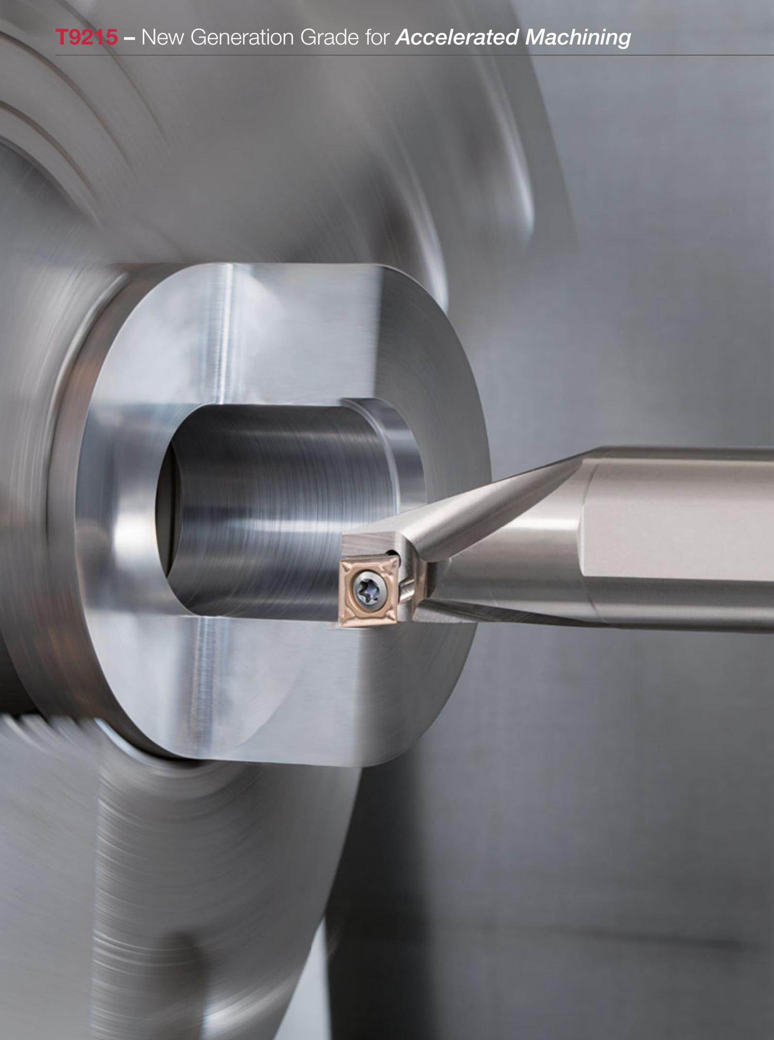
In external turning of shaft parts, the competitor's insert could machine only 1 pc per edge. Extended tool life with optimum cutting conditions was required to increase productivity.
