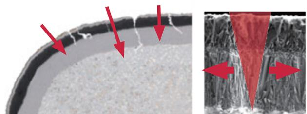
The crack gradually spreads
