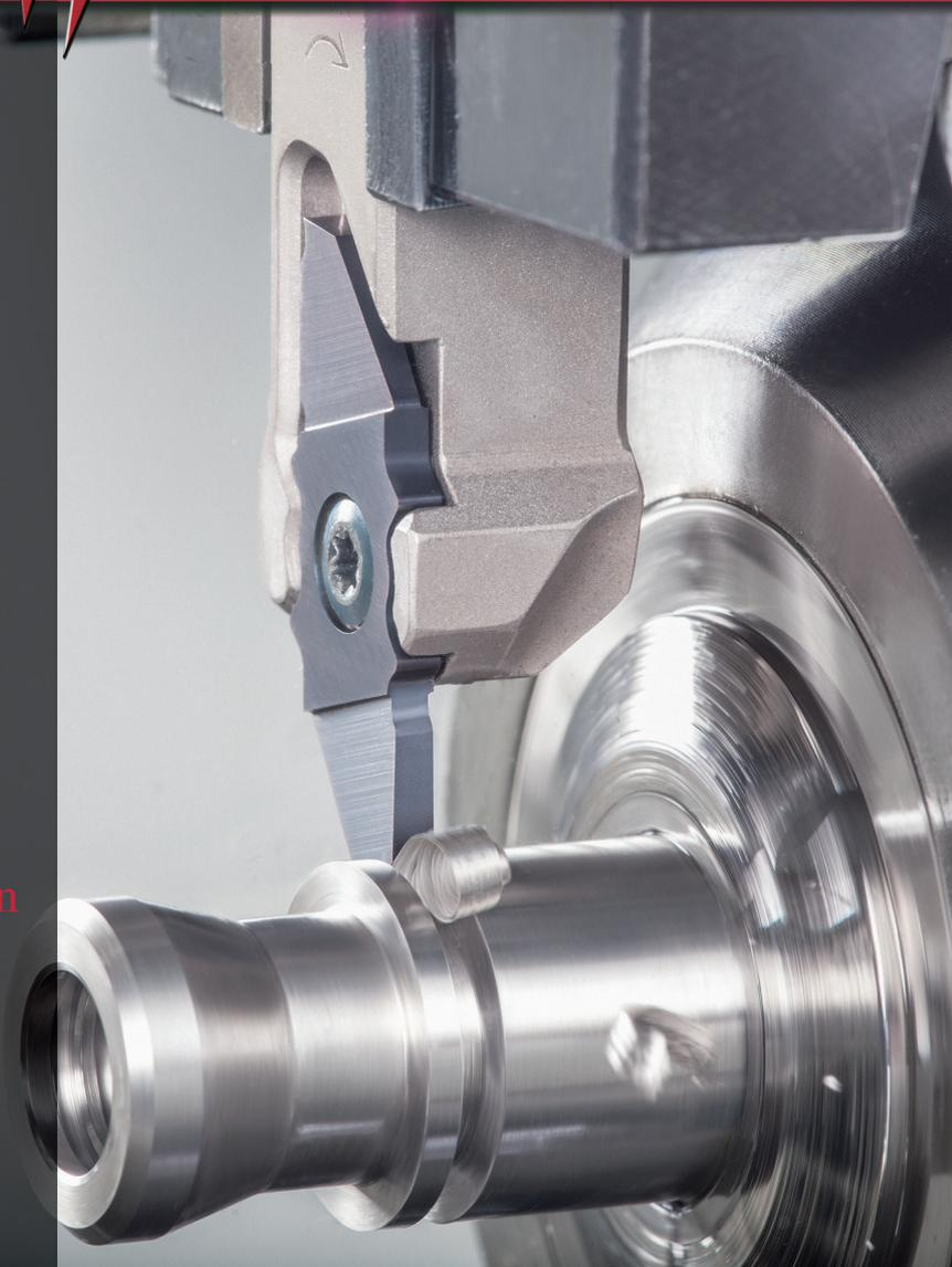
TungTech "DuoJust-Cut: Improves Productivity in Parting off Small Parts"
