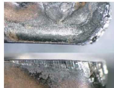
Increased flank wear leads to small chipping and welding
