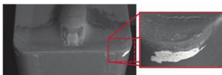
Tool wear after 30 grooves
