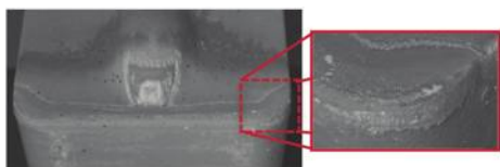
Tool wear after 60 grooves
