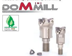
This is a cutter for semi-finish or finishing operation with profile milling or plunging. By using the double-sided inserts with a positive clearance angle, both the cutting edge strength and the sharpness have been realized. DoMiniMill endures high-feed milling, and the feed speed can be significantly increased by the combination with the multi-flute body.
