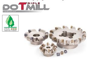
This face milling cutter has square, octagonal, and round inserts that can be fit in the same cutter body. The improved clamping structure reduces lifting of inserts and stress applied on the screws during heavy cutting.
